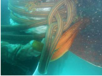
Figures 4.3.2.1/5 & 6: Underwater photos showing the entanglement of the towline at CHRISTOS XXII stbd propeller shaft
