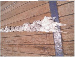
**Figure 4.3.2.1/8**: The end of the pennant's part that was affected by the shaft's and the blades' rotation.
