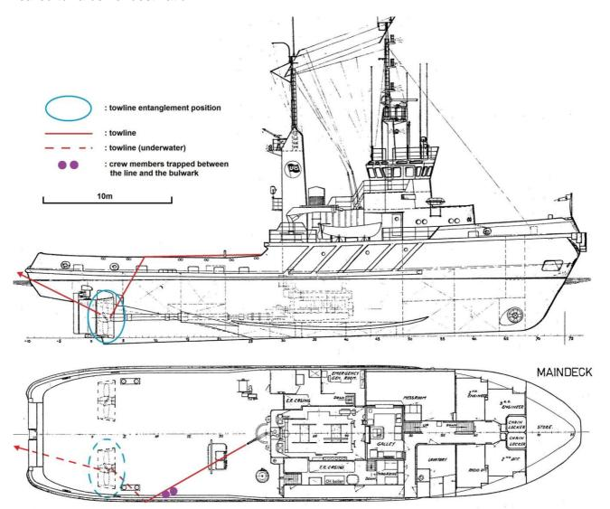
Figure 3.3/4: Depiction of the position of the towline and the trapped A/B and Motorman during the casualty.
