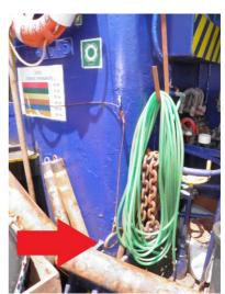
**Figures 4.3.3.1/2 & 3**: The towing hook quick release mechanism's wire route and handle are indicated by the red arrows.
