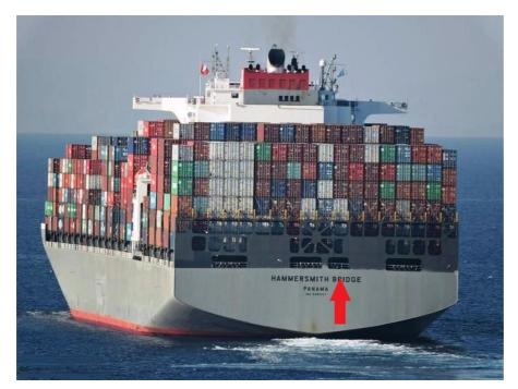
Figure 3.3/2: Indicative position (red arrow) of the towline's eye while being released by the HAMMERSMITH BRIDGE aft unmooring team and prior the exit of the T/B crew on its
