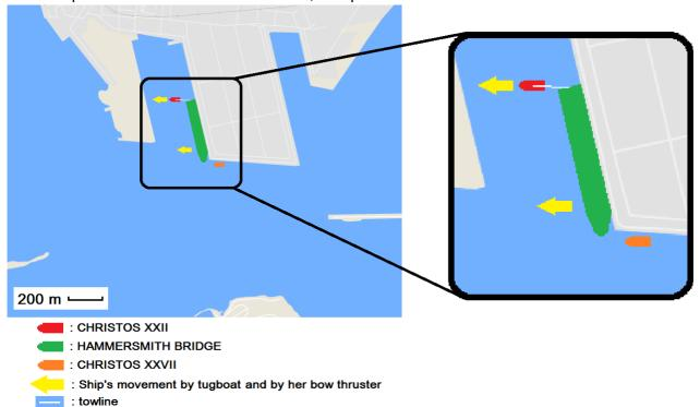
Figure 1/1: Intended towing procedure for the departure of HAMMERSMITH BRIDGE. Dimensions of the vessels and the towline are not scaled.
