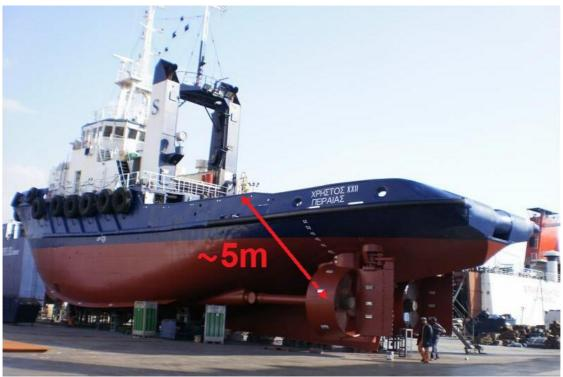
**Figure 4.3.2.1/4**: View of CHRISTOS XXII at a shipyard, showing the distance from the estimated point of the bulwark where the towline was taut until the propeller shaft (although the photo shows the port side of the tug, the same estimation stands for the stbd side as well).
