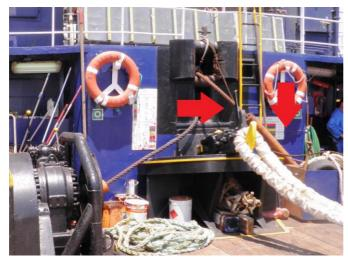
Figure 4.3.3.1/1: The towing hook quick release mechanism's wire route is indicated by the red arrows.
