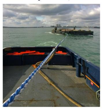
Figure 4.3.2.3/1: Indicative photo from a towage with the use of a gog rope (yellow color line) attached to a towline (blue & white color line). (Image Source: http://kingmarine.eu/tug-deckhand-course)
