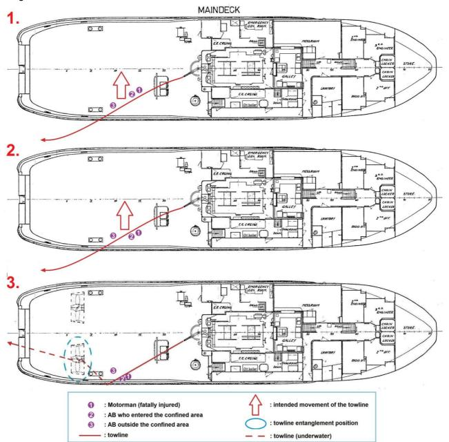
**Figure 4.2/1**: Phase 1: Pulling of the towline from all 3 crew members standing on its left side (looking forward).
