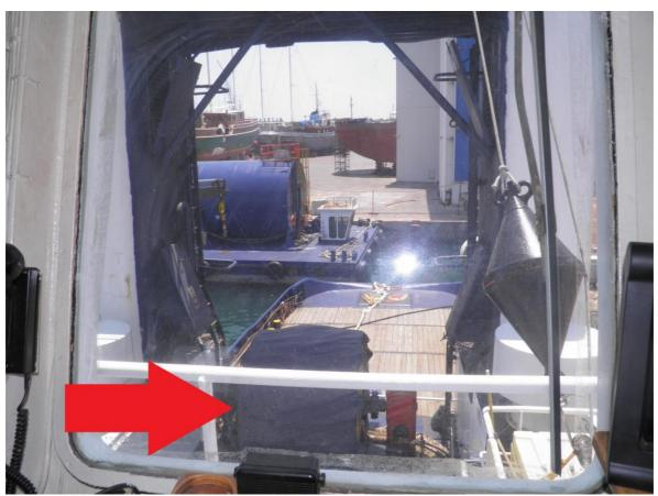
**Figure 4.6.3/1**: Astern view from the wheelhouse of CHRISTOS XXII. The red arrow indicates the position of the stowed equipment that blocked the view of the main deck stbd area.
