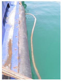
Figure 4.3.2.1/2: Part of the 40m Polyethylene fibre rope (orange color) floating at sea.
