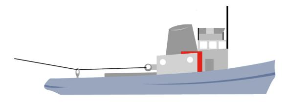
Figure 4.3.2.3/2: Side view of a T/B using a gog rope, showing its effect to the effective towing point.
