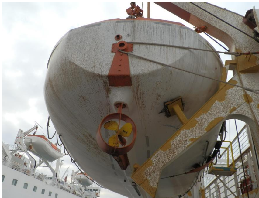
Figure 12: the same spray appears also on the life boat and its crane, which were nearby the port funnel (deck 8 port side)
