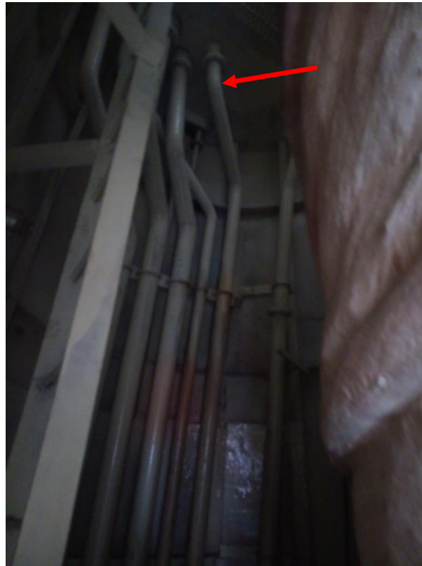
Figure 15: The air extractor pipe within the port funnel duct; capture is from underneath the panel where the air extractor pipe ends up (see indicator arrow and next figure). On the right side of the figure the main exhaust pipe is visible (photo captured after the repairs)
