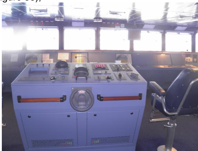
Figure 38. Helmsman workstation consoles.
