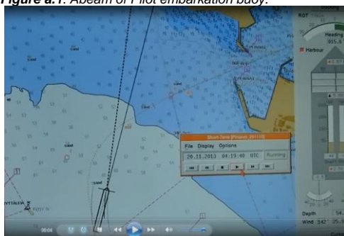
Figure a.3. Turning to starboard manoeuvre for bringing the bow into alignment with the port entrance.
