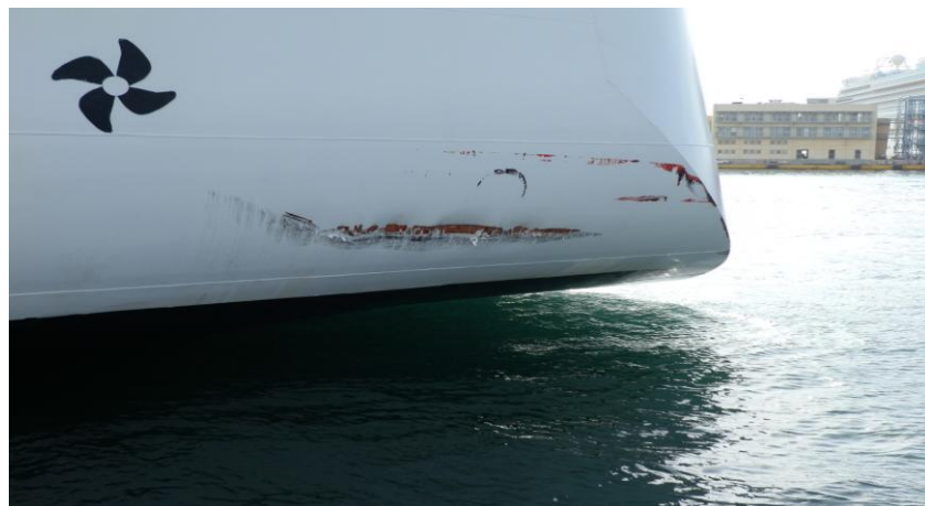
Figure 30. The sustained indent of port stern section caused by Tug Alexander III on the effort to push the stern section.
