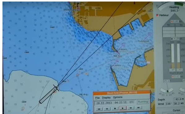
Figure a.5. Turning to starboard manoeuvre for bringing the bow into alignment with the port entrance.
