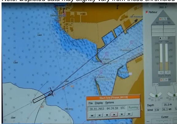
Figure B.1. Turning to starboard manoeuvre for bringing the bow into alignment with the port entrance.
