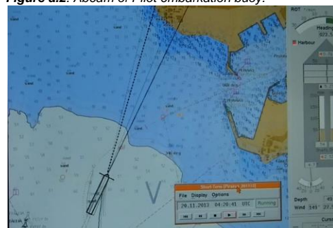
Figure a.4. Turning to starboard manoeuvre for bringing the bow into alignment with the port entrance.
