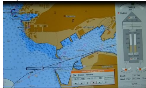
Figure d.2. Headway course-keeping manoeuvring towards port entrance.
