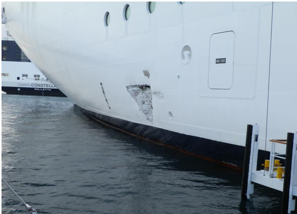
Figure 27. The damaged port bow section of MSC Magnifica.
