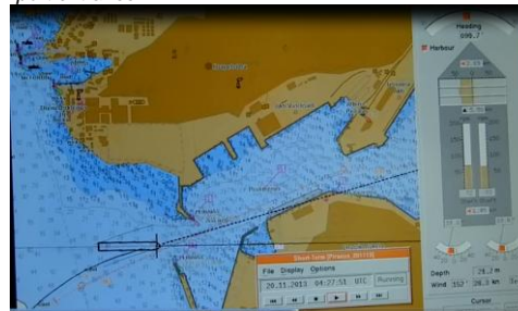
Figure d.4. Headway course-keeping manoeuvring towards port entrance.
