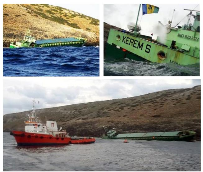
Figures 3.4/1, 2 & 3. Kerem S grounded at Levitha Island with a starboard list.
