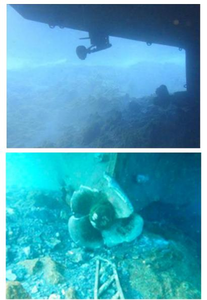
**Figure 3.2/1**. Missing rudder blade after the vessel's grounding.
