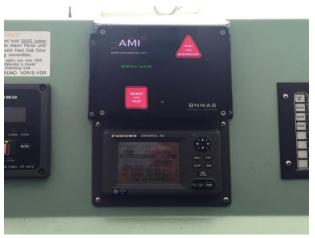
Figures 4.4.4.3/1 & 2: St. Gregory's BNWAS as presented in its Operational Manual and as fitted on board the vessel.
