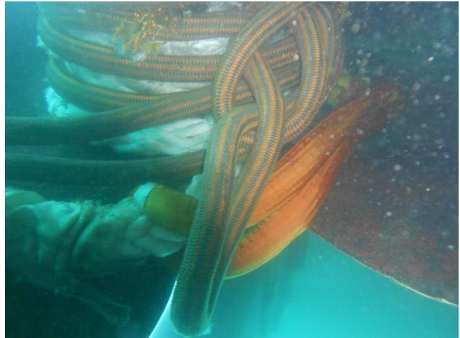
Figures 2,3: captures of the entangled rope on the tug boat's stbd propeller.
