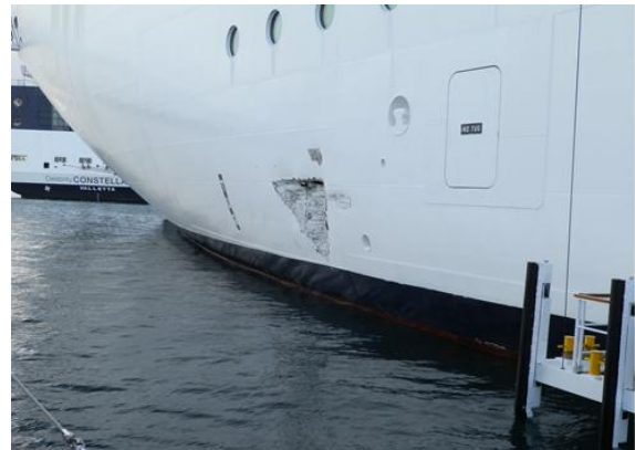
Figure 3: The damaged port bow section of MSC Magnifica
