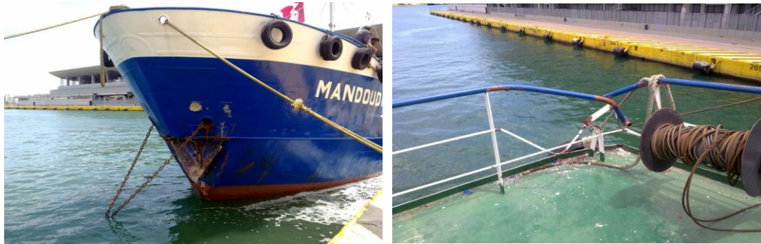
Pictures 2, 3: The damages of the M/T externally (left: fore part, right: railings on the starboard bridge deck)
