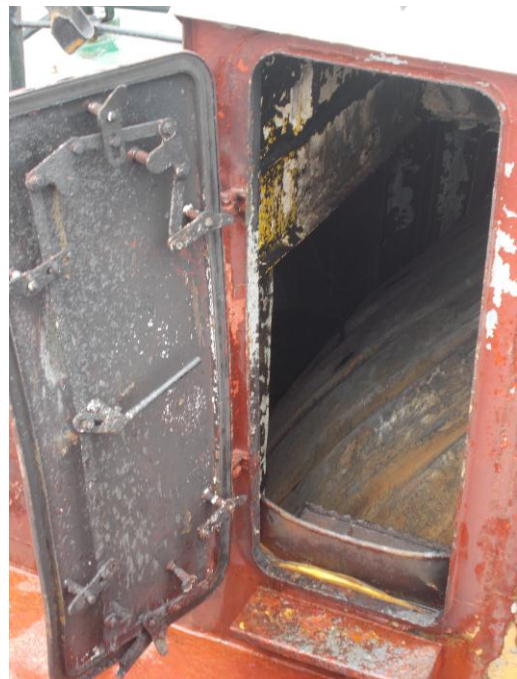
Capture of the cracked bulkhead of the Paint Room caused by the explosion.
