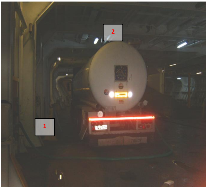
Picture 1: The tank truck parked near the water inlet valve, inside the garage of the Ro-Pax “NISSOS RODOS”. The water pipe, connected to the ship’s fresh water inlet valve is noticed. The position of the Boatswain (1) and the position of the driver (2) during the development of the accident have been marked.
