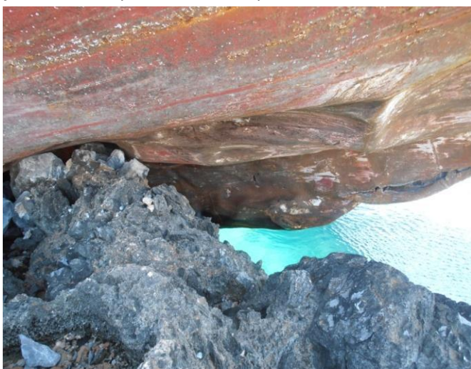
Deformed starboard fore bottom section.
