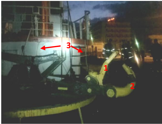
Picture 3: Arrangement of the quick release mechanism of ARTEMIS V. The releasing phases prior to activation (on the left) and past activation (on the right). 1: Hook fastening arm, 2: Towing hook, 3: Release wire from the coupled jointed arm to the bridge.
