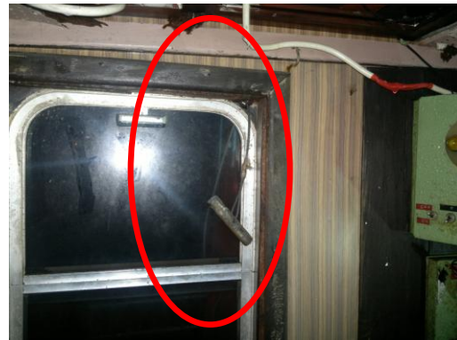
Picture 4: The lever release of the immediate release system of the tugs to the steering space of tug boat.
