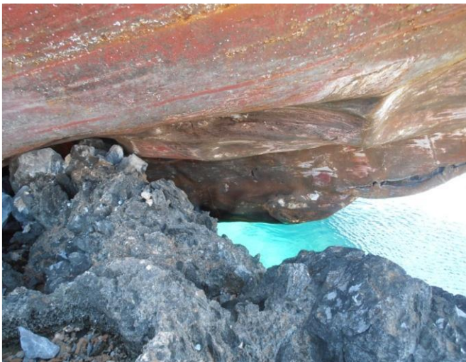
Deformed starboard bottom fore section.
