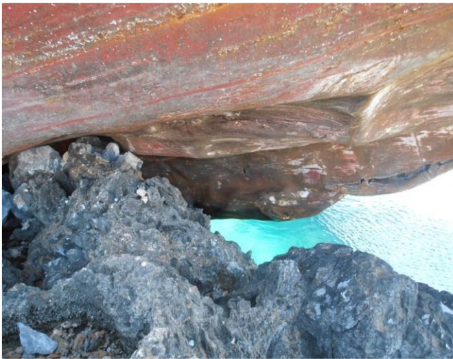
Deformed starboard fore bottom section.
