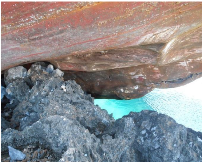
Deformed starboard fore bottom section.
