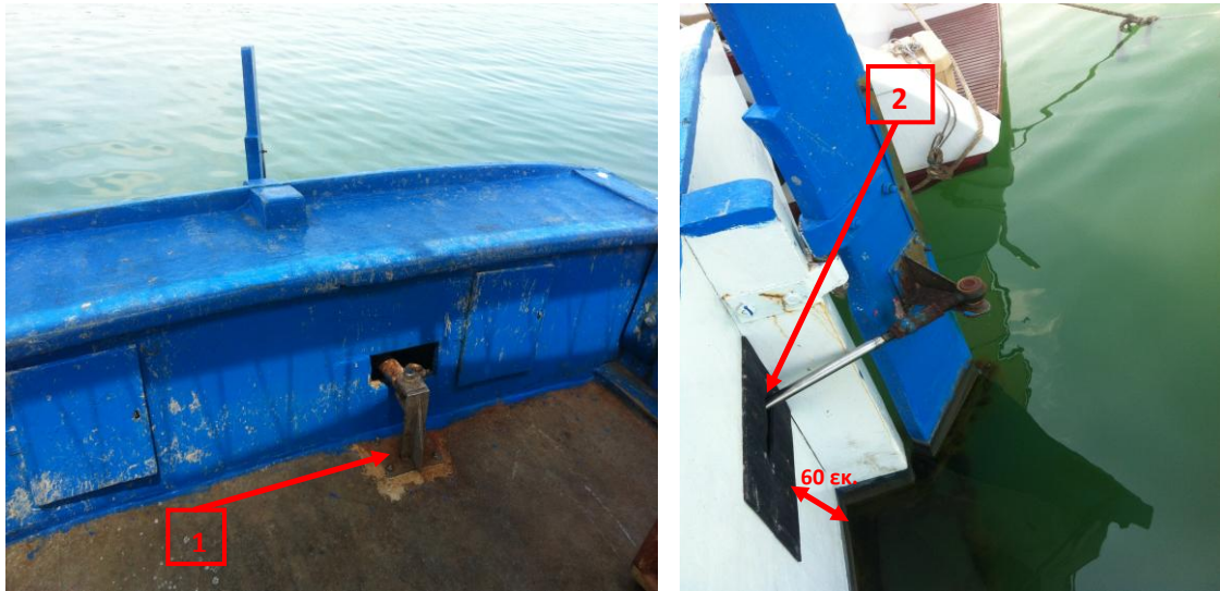
Picture 2: The bearing point of steering gear (1) and the point from which the rudder mechanism penetrated the hull of the ship (2).
