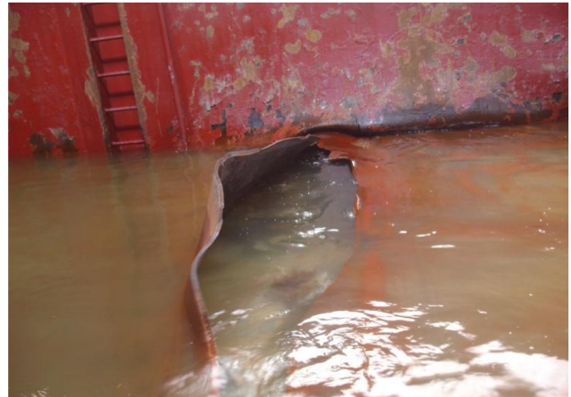
The crack at inner bottom plate of No 1 cargo hold.
