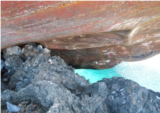
Deformed starboard bottom fore section.
