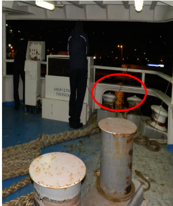
Picture 3: View of the left aft mooring deck space. Marked (circled in red color) the fairlead rollers through which the stern ropes passed which was the point where the seaman got injured.
