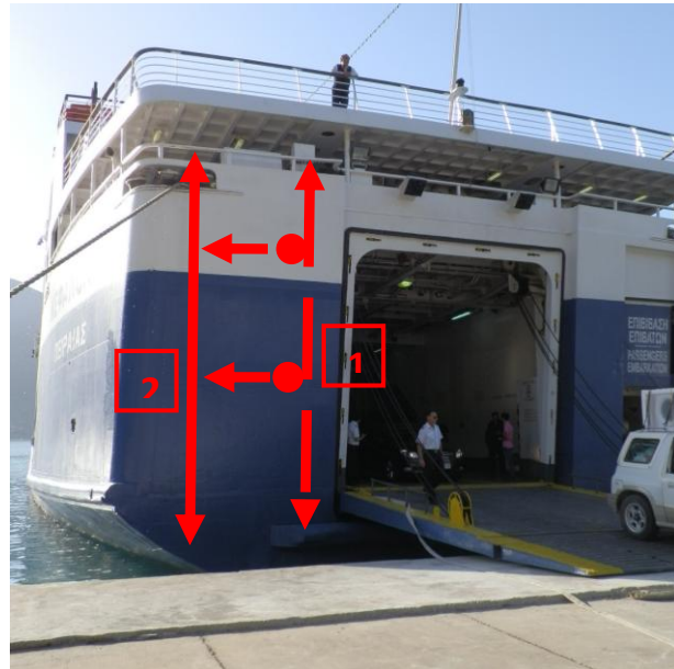
Picture 1: The initial (position 1) and final position (position 2) of the suspension of the rubber pad.
