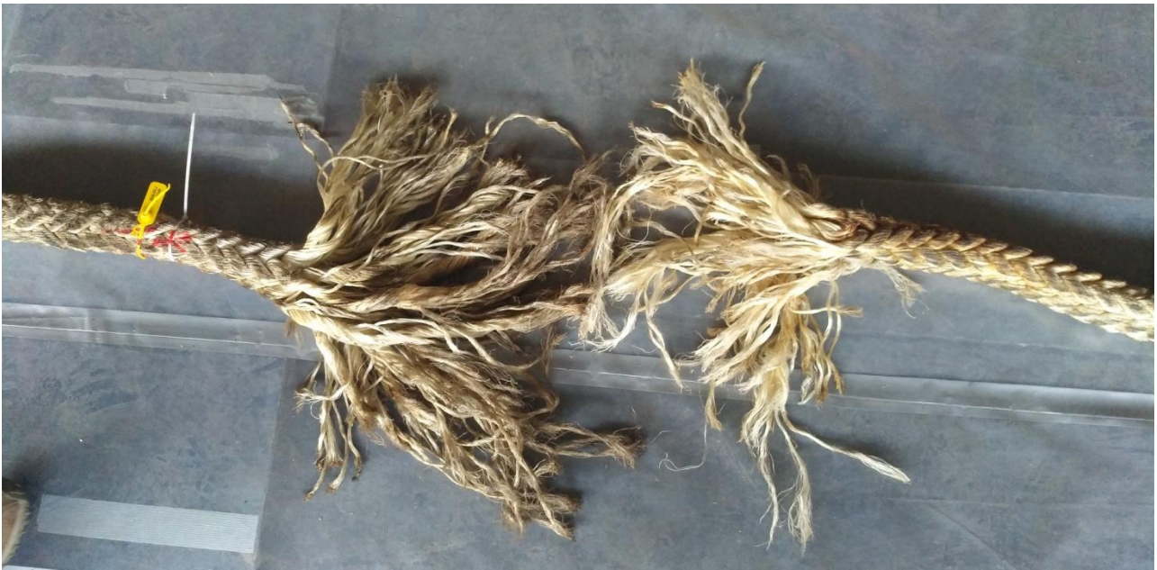
Figure2: The rope's breaking point at the part that remained onboard (left part of the photo) and at the part that remained on the terminal's bollard (right part of the photo).
